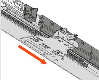
Fitting the driver pins to the runners
