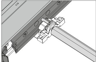
A pressure at any point on the drawer frontal is sufficient for the drawer to self-open
